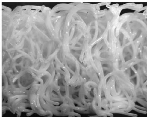
Figure 2. Breathair with complex fibers that produce a spring function (PU)
