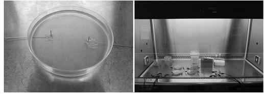
Figure 1. Experimental set-up; Left: petri dish with stainless steel electrode; Right: working in the biosafety cabinet
