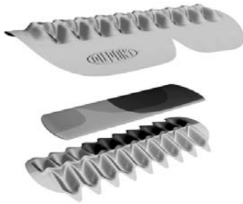
Figure 21: 'Impact wave'. Construction of the patented multi-layer protective fabric.
