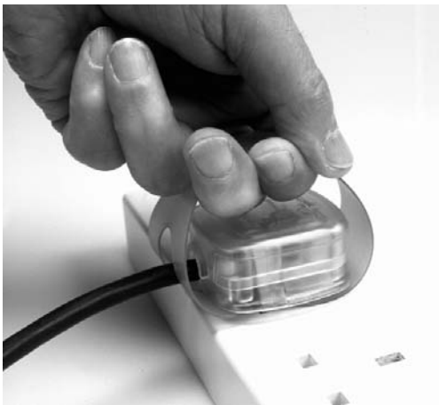
Figure 7. 'Pull the plug'. A simple, low-cost, colour-coded plastic strip that makes electric plugs easy to pull out. The coloured plastic strip meets current UK IEEE regulations and also makes for easy identification of plugs attached to different appliances. By Martin Bloomfield, RCA Industrial Design Engineering. Design for our future selves winner, 1999.
