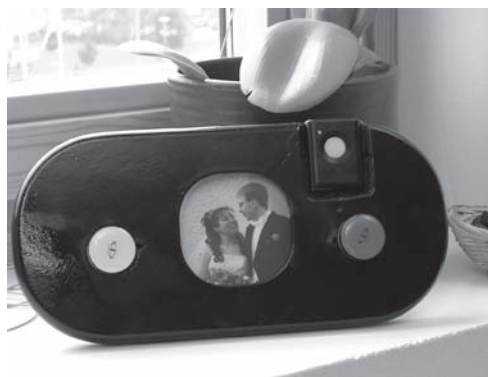
Figure 2. The first working prototype of the photo frame remote control with a small yellow on/off button, and large white and green browsing buttons to the left and right of the photograph
