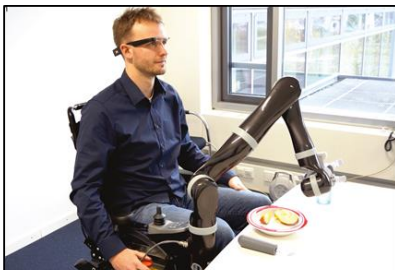
Figure 1 Scenario: User controls a robotic arm by head movements to eat and drink; Source: Own representation.
