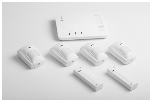
Figure 1. Picture of PIR, door/window sensors and gateway to internet router
